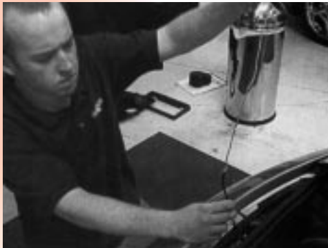
Routing the system wires.
