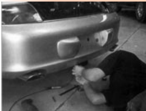
Installing the rear radar receiver.
