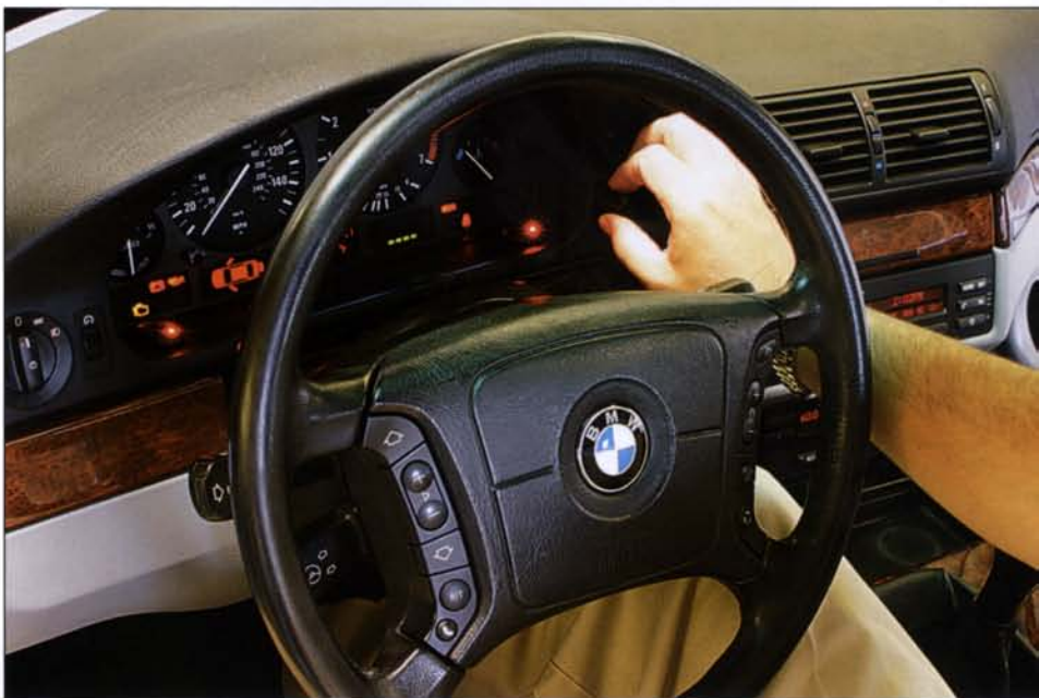
Two dime-size pods housing red LED warning lights are the heart of the system, attaching flush to the base of the instrument cluster and visually indicating power on and detected radar signals from the front or rear radar or front laser signal.
