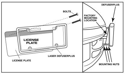
Note: For optimum performance, the DefuserPlus must be mounted parallel to the ground. Use the supplied K40 nylon nuts and bolts to correct the mounting angle of the DefuserPlus either up or down as needed.
