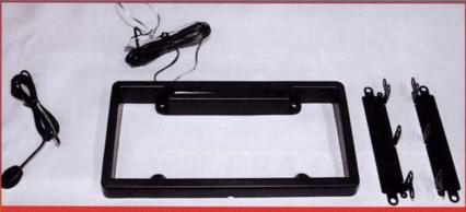
The kit comes with the DefuserPlus integrated into the license plate frame. The frame, however, didn't match the contours of our Mustang, so Topo Customs removed the unit from the frame and attached it to our existing license plate via one of the supplied brackets. The smaller window is the receiver portion of the DefuserPlus, and the wider side contains the diodes for the return jam.
