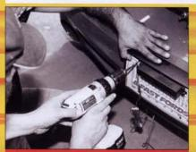
Camacho and Bob Biss add a mounting hole in the bumper through which we ran the wiring.
