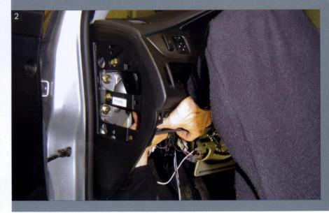
tion technology. A discrete radar receiver is mounted in the front and rear of the car. The receivers can be mounted behind the grill, or even behind the bumper as radar waves pass right through the plastic. Small dash-mounted LEDs and hidden piezoelectric speakers alert the driver of radar signals and a mounted rotary dial selects city / highway and controls volume.
