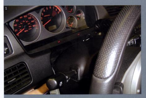
**1-2.** The most common location for the alert LEDs is the instrument cluster bezel. The bezel is first removed and then two small holes are drilled for LED installatio.
